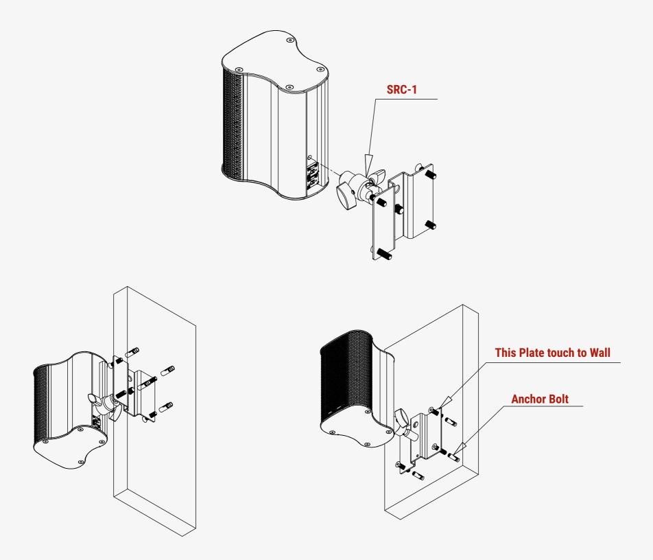
The illustration above displays the wall mounting arrangement for the ST 23 loudspeaker and identifies the essential hardware supplied.
